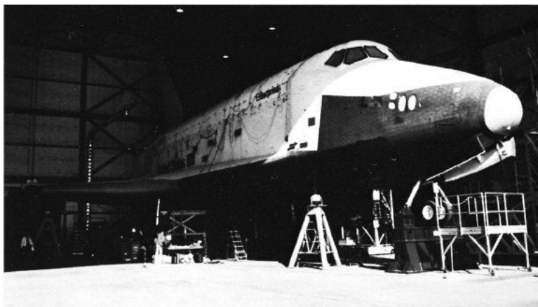
FIGURE 1.8 Vibration testing of the space shuttle Enterprise . (Courtesy of NASA.)
